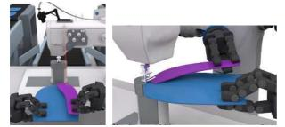
\*The image above is a proof of concept that is currently in development Sewing via a robot with an onboard visual recognition system
