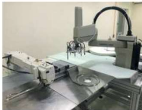
Fully automatic driver airbag sewing station
